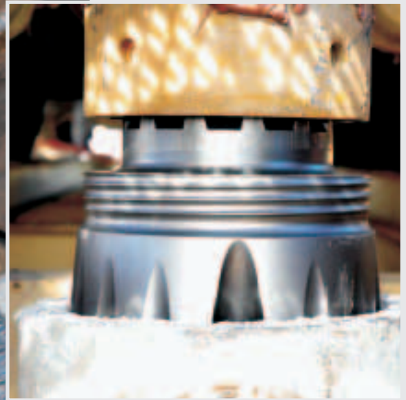
The dependable Atlas Copco Secoroc QL 120 with a 12 1/2" (318 mm) bit at the start of the drill run.
